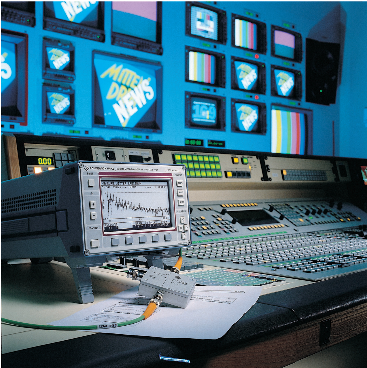
Digital Video Component Analyzer VCA for analysis of digital studio signals (photo 42246-1)
