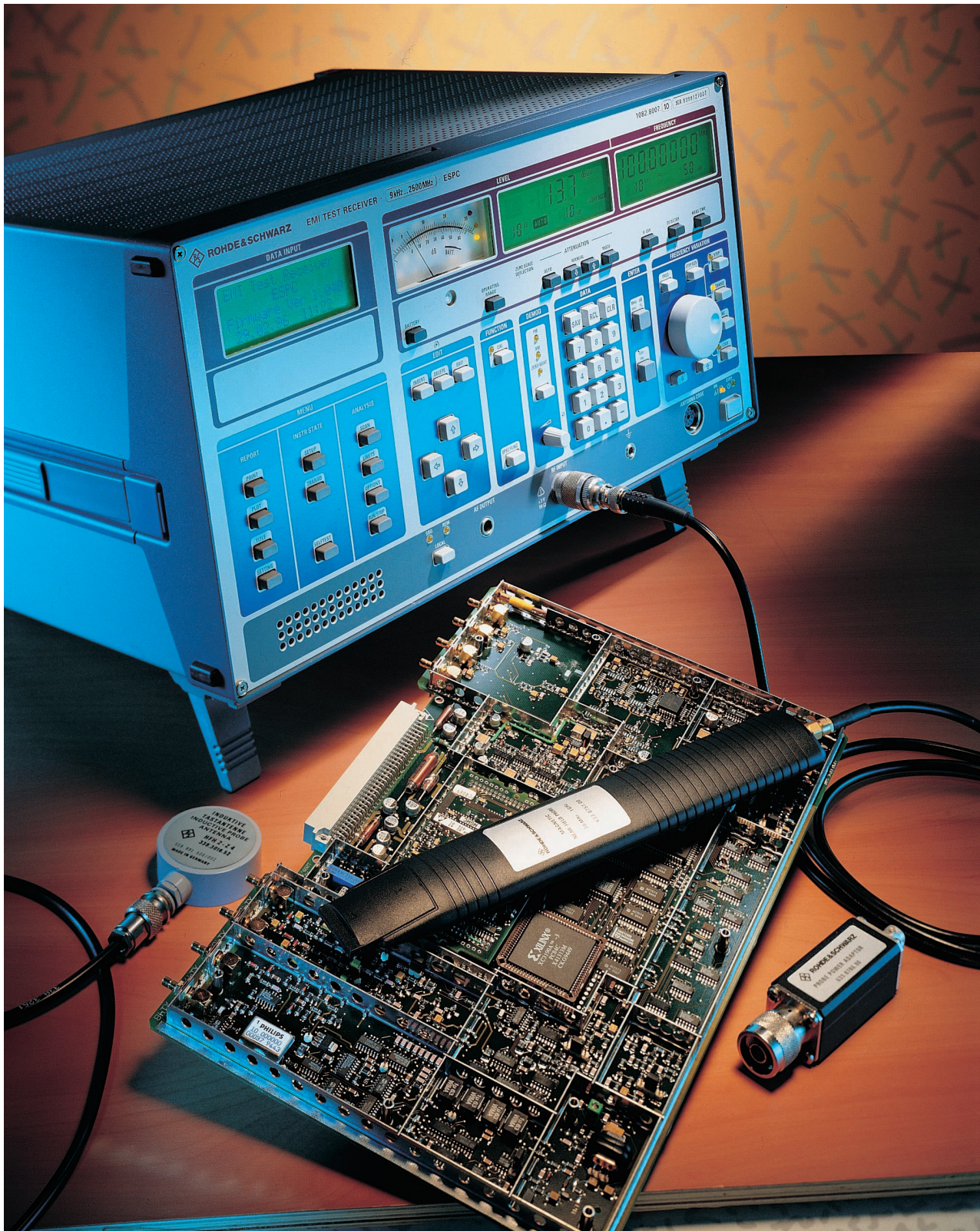
EMC pre-certification measurements with EMI Test Receiver ESPC and Near-Field Probe Set HZ-14 (photo 42446-1)
