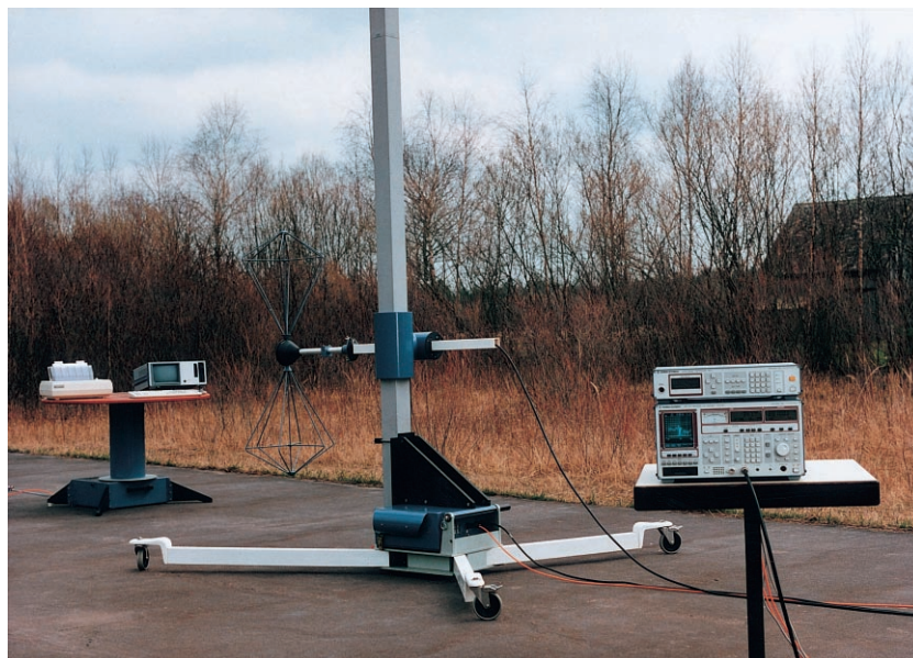
HCT12 with EUTs (left), HCM with antenna and HCC on top of test receiver (photo 40407-5)
