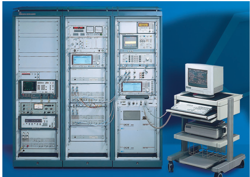
Test System TS8915B with audio option for all GSM standards (photo 42284)
