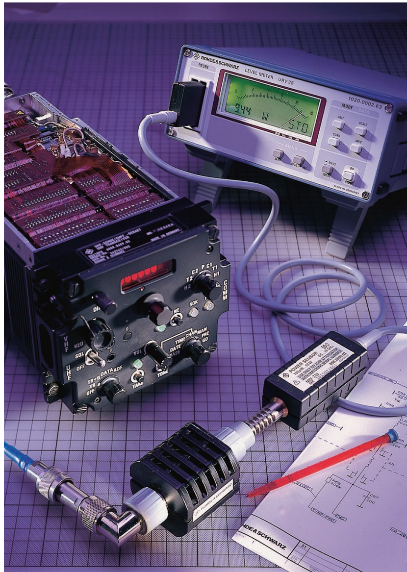
Output power measurement of a UHF transceiver with NRV-Z53 and URV-35 (photo 41 057)
